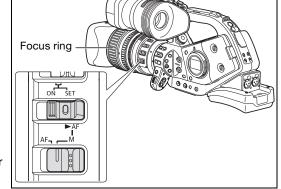
focus is a result of the internal temperature rising in the camcorder and lens. Check the focus before resuming shooting or adjust the flange back as necessary ( 28).
